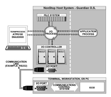
To communicate with the 6530, your application makes calls to the Guardian file system requesting various I/O operations, such as reads and writes. These calls access a set of generic procedures used to perform I/O on different types of devices as well as files. The workstation or PC is treated as a system terminal. The use of generic procedure calls for I/O makes most of the device-specific details transparent to your application.
